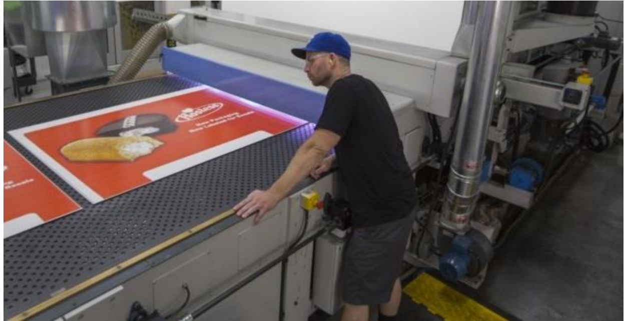
Digital corrugated printing in action at Bennett Packaging. Image courtesy of Bennett Packaging via Packaging Impressions.
