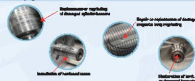
As part of the rebuild precess, we will completely refinish the curious of the sylinder. Also, there is an important management and the sylinder being resonantified. All new boartess are installed to everufacturers appealisations to ensure proper its and present proventure follows.
